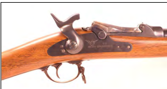
c) Half cock position (used to open breech).
